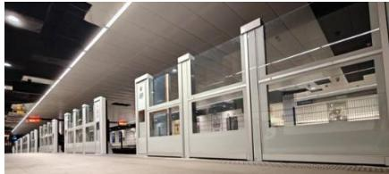
The modernisation of the Glasgow Subway continues. The full fleet of new trains have been in service for some time, and recently platform screen doors have been erected at some stations (first was Govan, photo from X/Twitter) in preparation for the introduction of 'driverless' trains, which will initially see drivers remain until the system has been fully proven.
